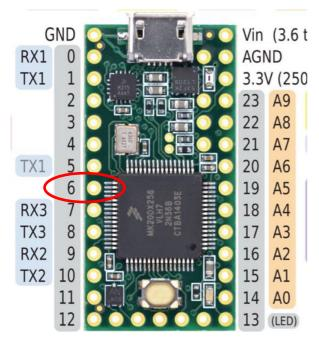
IMPORTANT! You are connecting a jumper wire to PIN 6 of the Teensy 3.2.
