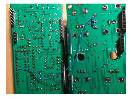
The update involes using an ON-OFF-ON switch instead of ON-OFF (or replacing if updating a current build), installing a <del>100K</del> 33K resistor, and adding a jumper wire between boards. Locate the range switch on the PCB.
