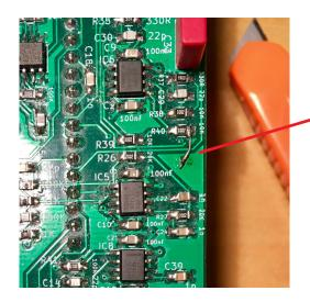
Solder a small wire or resistor leg to connect R40 to ground.
