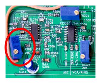
TR302 adjusts the radio AGC output level. Make sure the DIRECT/OD/AGC switch is set to AGC
